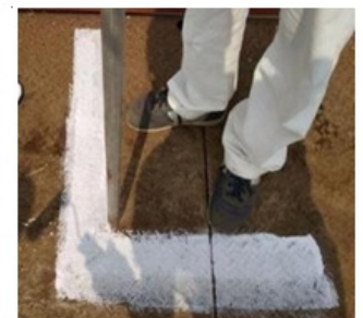
Figure: Sample GCP, placement on ground and taking reading on it
